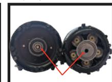
5. Locate the straight spot on both the motor and replacement head. These parts will mate with each other.
