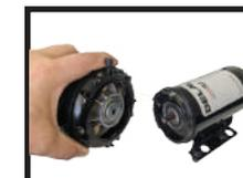
4. Twist and remove the pump head from the motor body.
