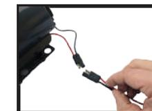
1. Disconnect electrical connections to pump.
