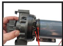
6. Place pump head on shaft of motor and rotate until the set screw holes are beside each other as shown above.
