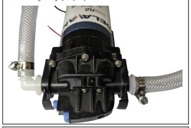
4. Next set the Bypass . Close the outlet side of the pump to pressurize the hoses and stop all flow (this is often done by hooking up your wand and stopping the flow). Using a 1/16" Allen key turn the bypass set-screw until it reaches 100 PSI.
