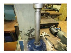
a. Flip end plate over and press the seal in next. The viton (rubber) lip should be facing the tool being used to press it in (or facing the inside of the pump).
