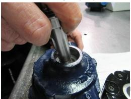
a. Using a hollow inside 1.5" outer diameter press tool, press on the outer race of bearing in until reaches the bottom of the bearing bore.
