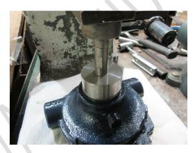
c. Insert the rounded end of the shaft (not the side with the keyway machined in it) through the bearing and seal and towards the inside of the pump.
