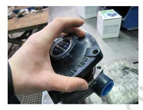
25. Once the end plate is back onto the rest of the pump replace the 4 bolts. Tighten bolts in a diagonal pattern from one corner to the opposite corner. (Follow order below)
