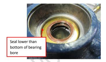
b. Using a 2.0" diameter press tool, press on the outer race of the bearing until it bottoms out on the bearing bore.
