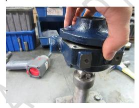
6. Now that the end plate is removed flip it around and push the nameplate out of its place from the inside.
