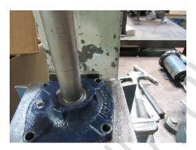
8. Using a ¾" diameter press tool press the new bearing in first. With the front of the end plate (side with lettering) facing up, press the bearing into the end plate with the lettering on the bearing facing towards the press tool, until the front of the bearing is flush with the face of the endplate.
