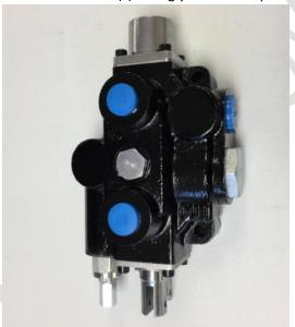
2. Locate the large Bung Fitting on the right-hand side of the valve body and remove it using the 1 1/2" wrench.
