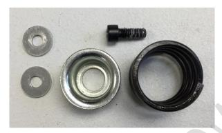
4. Install the detent assembly onto the spool shaft. Apply blue Loctite on the threads of the detent assembly. A screwdriver may be used to tighten the detent assembly via the large end slot.
