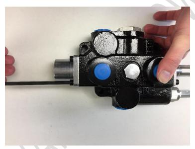
2. Remove the spool positioner assembly. If the handle is not installed, use a screwdriver to keep the spool shaft from rotating.
