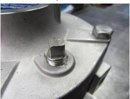
6. Spray a light oil into the ports of the pump and spin the shaft to coat as much of the inside surfaces of the pump as possible to aid in avoiding corrosion.
