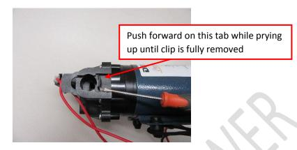
a. Replace slide connector clips with clips supplied in fittings pack. Make sure that the larger of the two holes in the clip is pointed to the back of the pump, and the side of the clip that has the small notch in it, is facing the center of the pump.
