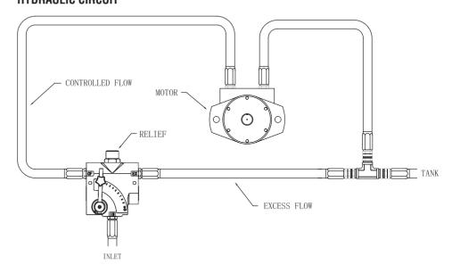
HYDRAULIC FLOW CONTROL VALVE WITH BELIEF
