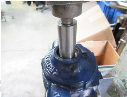
16. Next, use a 1.2" diameter press tool to press the new body seal back into the body of the pump. It is critical the seal is pressed below the lip that is designed to stop the bearing once it is pressed deep enough. If the seal is not pressed far enough down the pump will not spin freely and this could result in a damaged seal.
