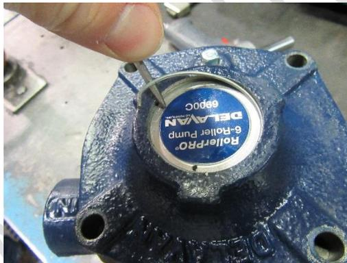
10. The end plate is now rebuilt and may be set aside until final assembly.
