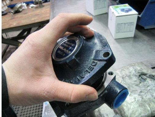
25. Once the end plate is back onto the rest of the pump replace the 4 bolts. Tighten bolts in a diagonal pattern from one corner to the opposite corner. (Follow order below)
