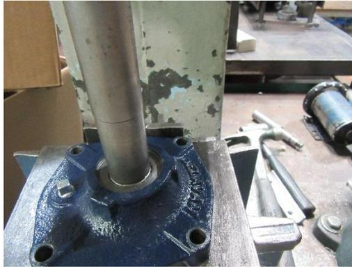
8. Using a  $\frac{3}{4}$ " diameter press tool press the new bearing in first. With the front of the end plate (side with lettering) facing up, press the bearing into the end plate with the lettering on the bearing facing towards the press tool, until the front of the bearing is flush with the face of the endplate.
