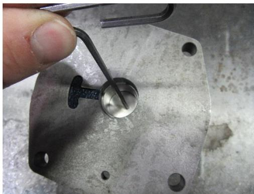
7. Once the name plate is removed the seal and needle bearing need to be pressed out using a  $\frac{3}{4}$ " press tool and replaced with the new bearing and seal. (If you do not wish to replace the needle bearing you may pry seal out with prying tool and replace with new seal using  $\frac{3}{4}$ " diameter press tool)
