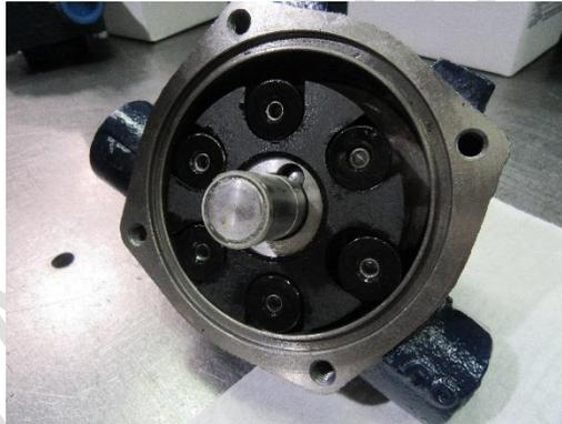
23. Add in new square seal ring if needed. (pry out using a pick, and replace with new)
