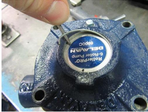
5. The end plate will need to be rotated so the edges can be pulled on to aid in removing plate.
