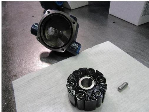
12. The bearing in the body of the pump is held in with a circlip that will need to be removed.
