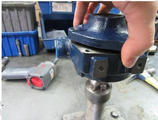
6. Now that the end plate is removed flip it around and push the nameplate out of its place from the inside.
