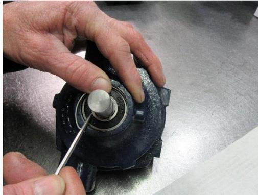
13. Press the shaft out of the body.
