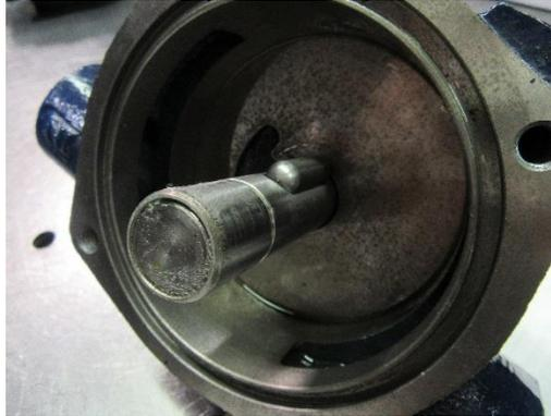
22. Slide the rotor onto the shaft, then replace the rollers. The rollers can go in either way and will not affect the performance of the pump.
