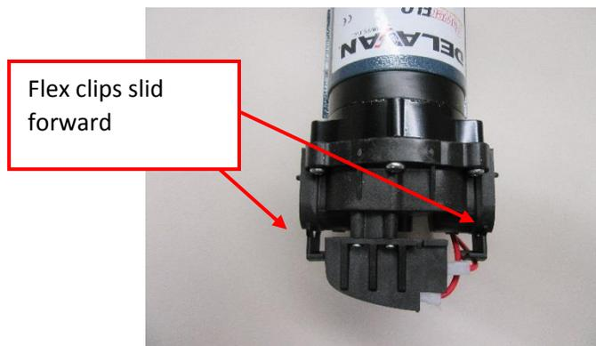
3. Next, take the small flat blade screw driver or similar tool, and pry the back of the clip (closer to the motor) away from the center of the pump and push forward on the clip until it comes off the pump. Repeat for opposite side.
