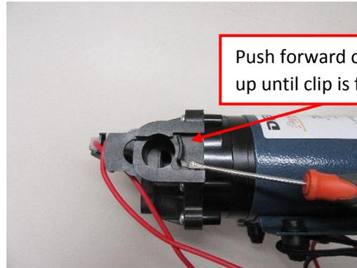
Push forward on this tab while prying up until clip is fully removed
